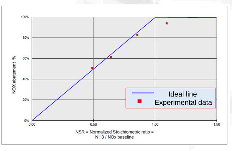
Ammonia consumption in a SCR application is very close to the reaction stoichiometry. Ammonia is almost absent at the stack, apart those periods when the line is operated in direct mode, when ammonia is not captured in the milling phase and appears at the stack (around  $18 \text{ mg/Nm}^3$   $10\% \text{ O}_2$ )
