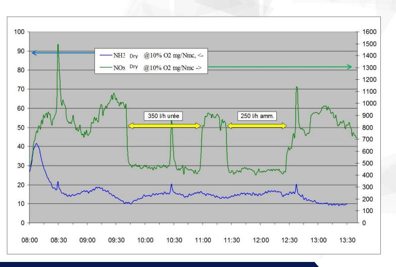
In these kind of applications the reduction efficiency is in the order of 40%; starting from emission levels of 800 mg/Nm<sup>3</sup> it is consequently possible to stay below 500 mg/Nm³, without ammonia slip, both using urea or ammonia solution.
