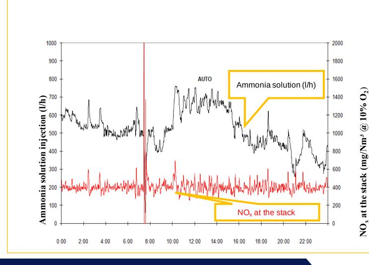
The application of SNCR technology to the precalciner produces much better results, provided that an even distribution of the reagent is realized and oxidizing conditions are guaranteed.
