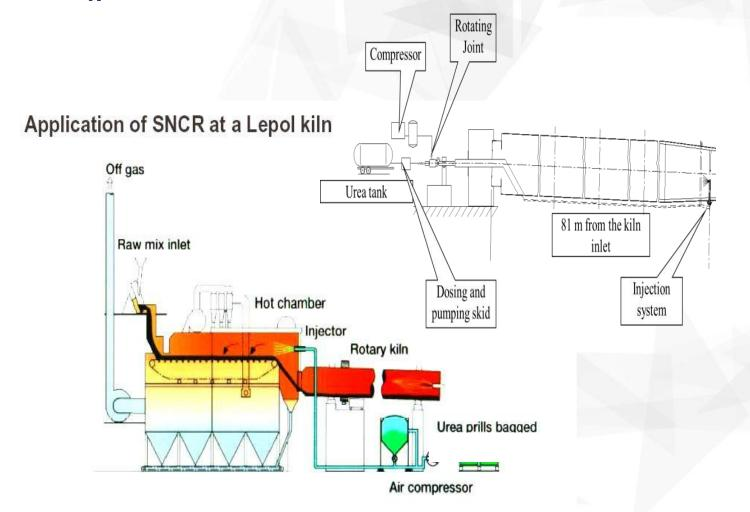
The second kind of actions is based on the reaction between amide NH<sub>2</sub> and NO, to form nitrogen and water, this reaction can take place spontaneously at around 900°C, or catalyzed by Ti and V oxides at 300-350°C. The first technology, the Selective Non Catalytic Reduction (SNCR), has been applied to almost all kind of kilns, trying to inject urea or ammonia solution where the best temperature window is located.
