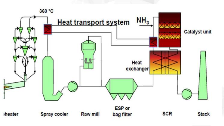
The SCR technology can be also applied as a tail end system (low dust SCR).
